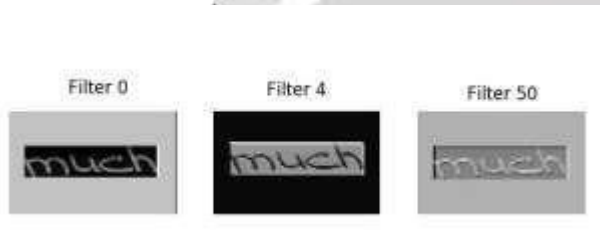
Figure 3. These are the filters from the first convolutional layer of the RESNET-18 word segmentation model with the example word "much"
